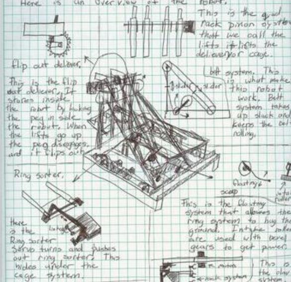
Labels in diagram: Flip out deliverer, Ring sorter, Drive train, Claw, Lock and Load, Ring sorter, Flip out deliverer, Ring sorter, Drive train, Claw, Lock and Load.
